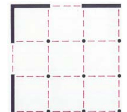
Minimization of Load Bearing Walls
